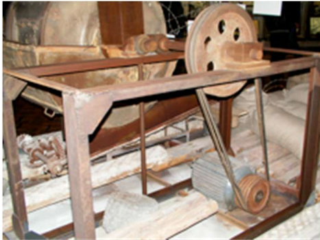
Fig. 12: Electric motor operating the Yanov mill Photograph: Private, Kiev 2011.
